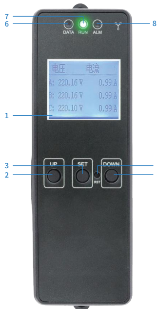
Three-phase PDU meter panel display
