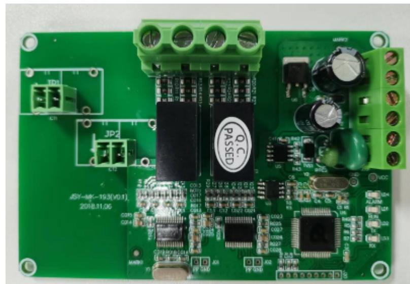
2.2.1 The working power supply of the module can be selected, DC 9-30V
